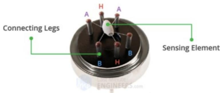
**Figure 2.** MQ2 Sensor, Inside View. Source: <https://lastminuteengineers.com/mq2-gas-senser-arduino-tutorial/>}}
