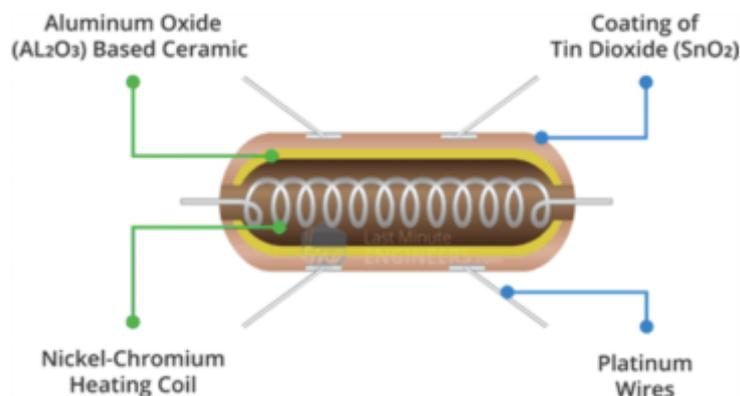
**Figure 3.** MQ2 Sensing Unit. Source: <https://lastminuteengineers.com/mq2-gas-senser-arduino-tutorial/>}}
