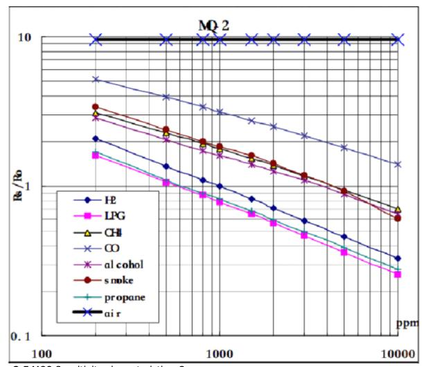
**Figure 2.5** MQ2 Sensitivity characteristics. Source: https://www.mouser.com/datasheet/2/321/605-00008-MQ-2-Datasheet-370464.pdf}}
