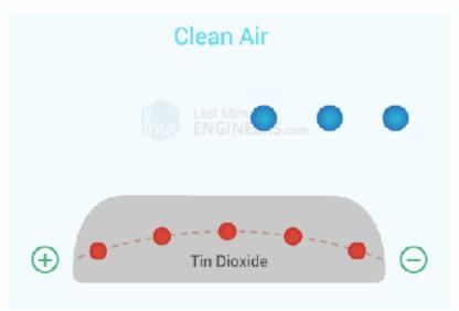
**Figure 2.4** Chemical process altering the resistance in the module which causes a change in voltage output. Source: <a href="http://lastminuteengineers.com">http://lastminuteengineers.com</a>}
