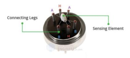
Figure 2.2 MQ2 Sensor, Inside View. Source:
