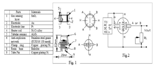
Figure 2.1 MQ2 Sensor Schematics. Source:
