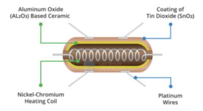
Figure 2.3 MQ2 Sensing Unit. Source:
