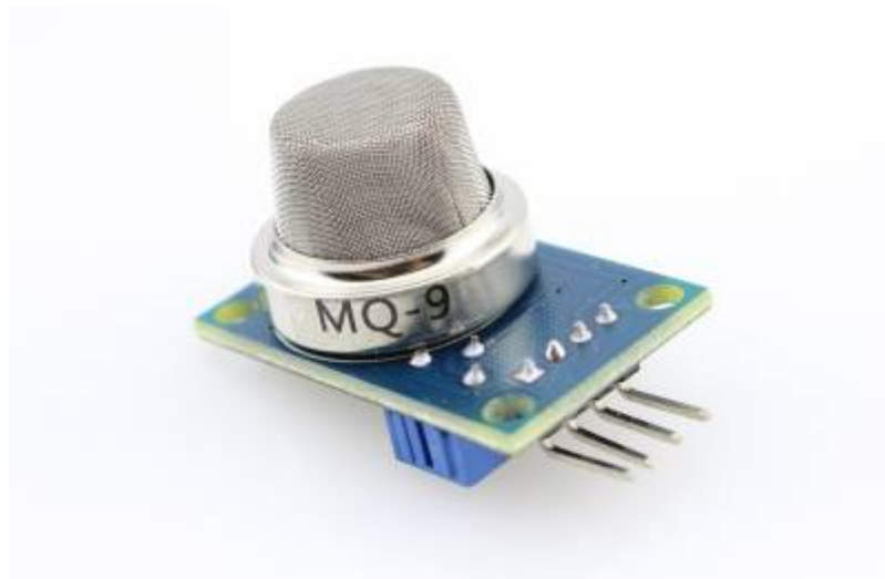
Figure 1 MQ9 Sensor. Source: https://www.instructables.com/How-to-Calibrate-Use-MQ9-Gas-Sensor-W-Arduino/
