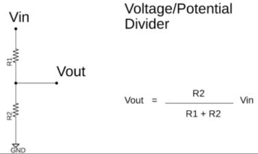
**Figure 4** Source: https://www.electroniclinic.com/what-is-a-voltage-divider-or-potential-divider-formula-and-practical-uses/
