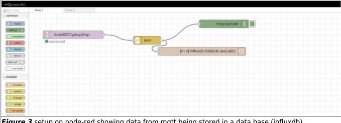
Figure 3 setup on node-red showing data from mqtt being stored in a data base (influxdb)
