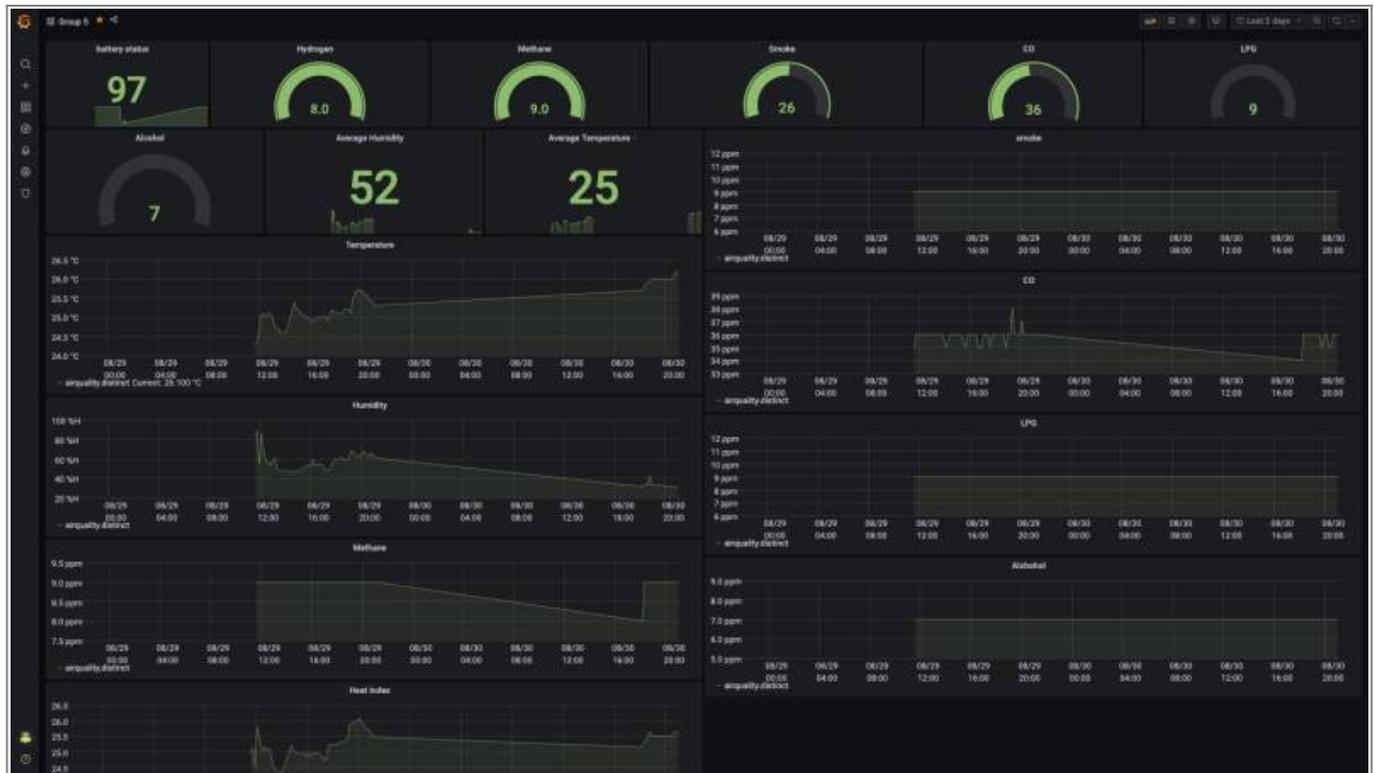
**figure 7** Measurement result of DHT22 and MQ2 sensors visualized on Grafana
