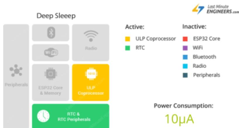
**Figure 5** ESP-32 Active Components during Deep Sleep mode. Source: <https://lastminuteengineers.com/esp32-sleep-modes-power-consumption/>
