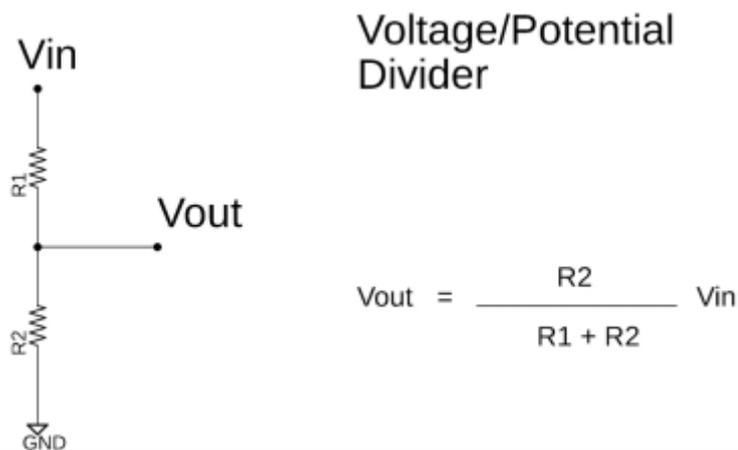
Figure 4 Source: <https://www.electronicclinic.com/what-is-a-voltage-divider-or-potential-divider-formula-and-practical-uses/>
