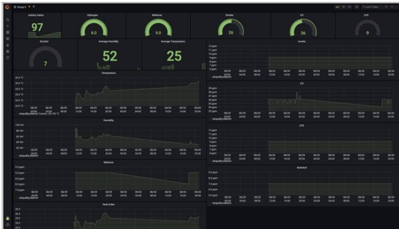
figure 7 Measurement result of DHT22 and MQ2 sensors visualized on Grafana
