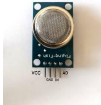
Fig. 3: MQ135 sensor Module (Taken by Emilie Streichsbier)
