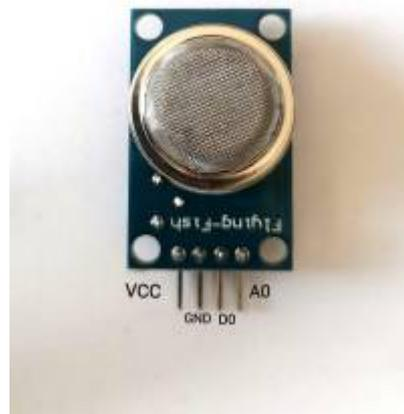
Fig. 3: MQ135 sensor Module (Taken by Emilie Streichsbier)
