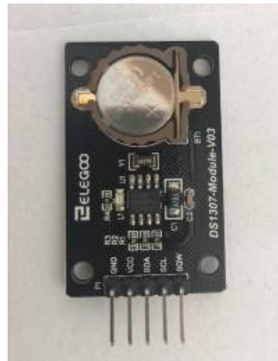
Fig. 4: RTC DS1307 Module (Taken by Emilie Streichsbier)
