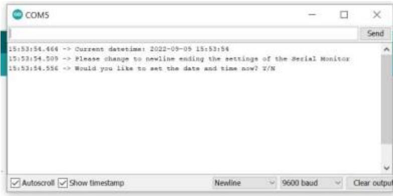
Fig. 5: Setting the time in the serial monitor
