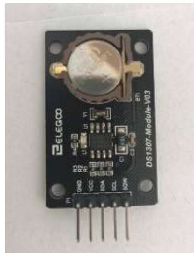
Fig. 4: RTC DS1307 Module (Taken by Emilie Streichsbier)
