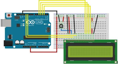
Fig. 1: LCD Set-up (Source:
