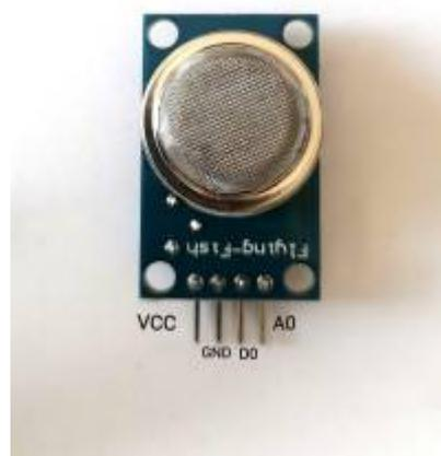
Fig. 3: MQ135 sensor Module (Taken by Emilie)
