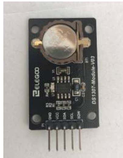
Fig. 4: RTC DS1307 Module (Taken by Emilie Streichsbier)
