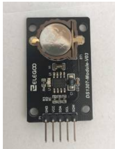
Fig. 4: RTC DS1307 Module (Taken by Emilie Streichsbier)
