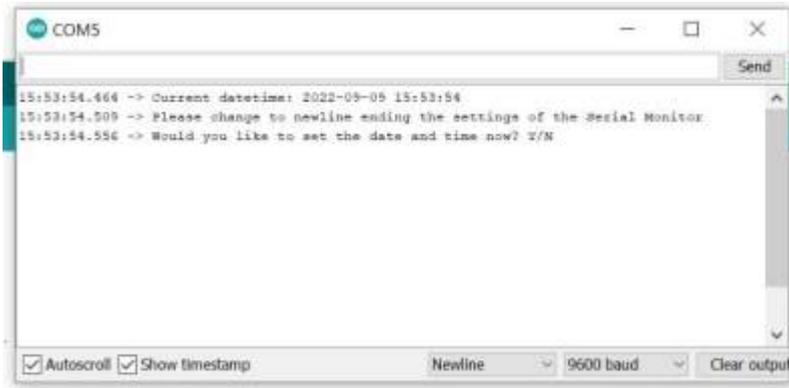
Fig. 5: Setting the time in the serial
