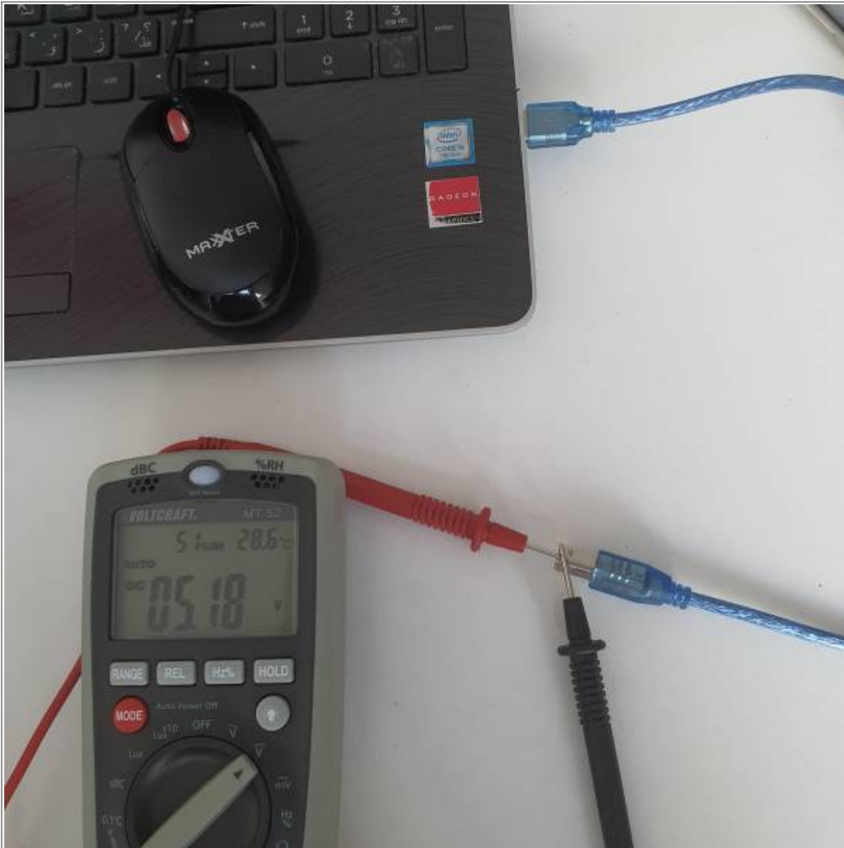
Figure 20 Measuring the voltage supplied by the Laptop USB port directly, Photo by Ziad Helou
