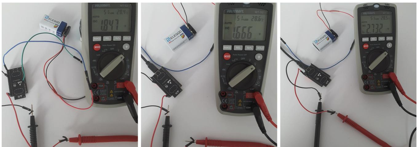
In the three schematics, the maximum voltage supplied from the ESP32 to the sensors was 2.73 volts, which is also insufficient to power our sensors. 2.73 volts was the best voltage reached when using the battery in all our trials when connecting the battery using the micro cable USB as input and the 5V pin as output.
