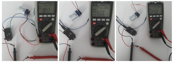
In the three schematics, the maximum voltage supplied from the ESP32 to the sensors was 2.73 volts, which is also insufficient to power our sensors. 2.73 volts was the best voltage reached when using the battery in all our trials when connecting the battery using the micro cable USB as input and the 5V pin as output.
