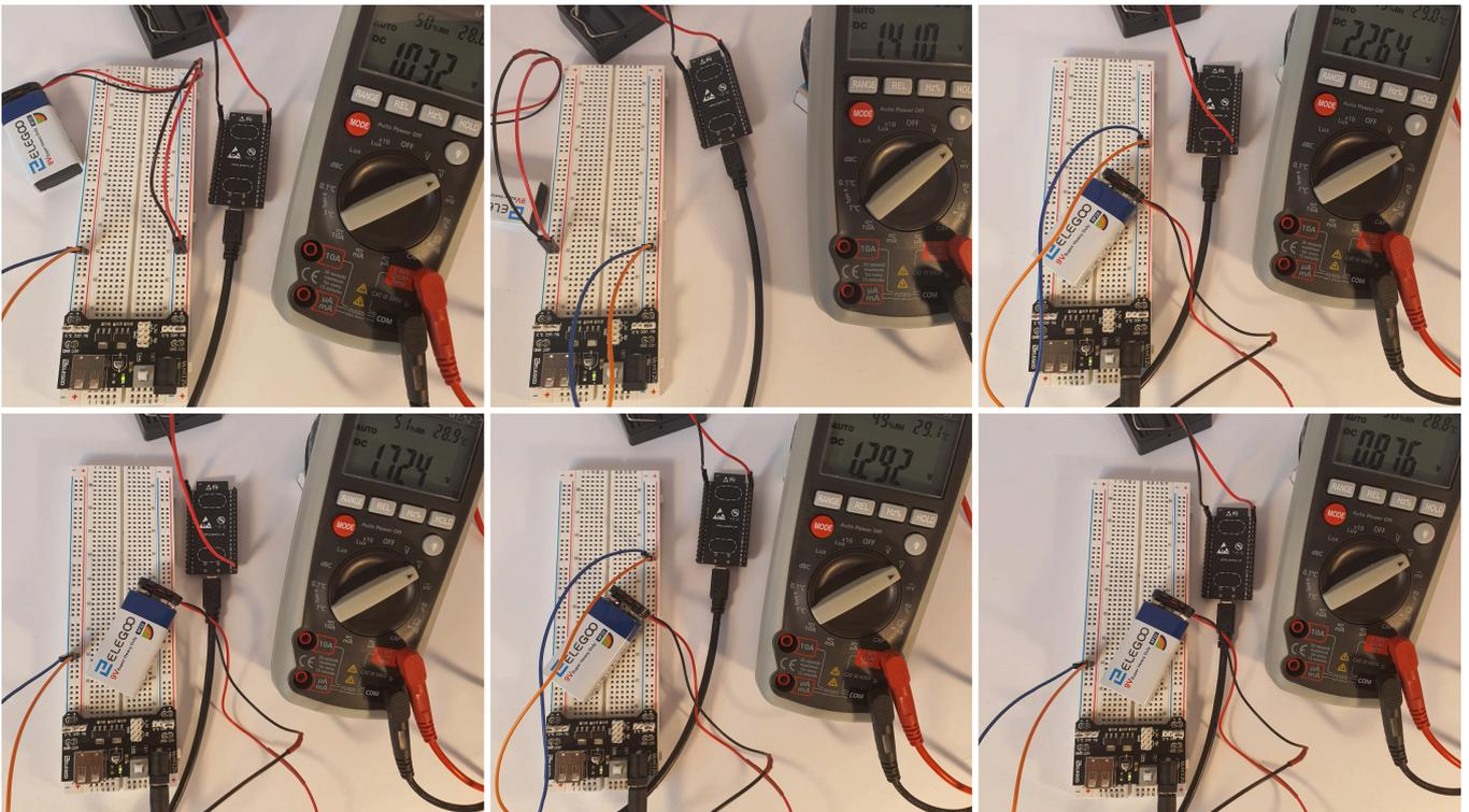
it is shown how we tried to work on many schematics using the 3V3 volts in the power supply or the 5V. The power supply is linked to the ESP32 using a micro cable USB or the 5V pin as an input. When using the micro cable USB, also we had two options, one to use the pin 3V3 as output in the ESP32, and the other to use the pin 5V. In all options, the maximum voltage supplied from the ESP32 to the sensors was 2.2 volts, which is also insufficient to power our sensors.
