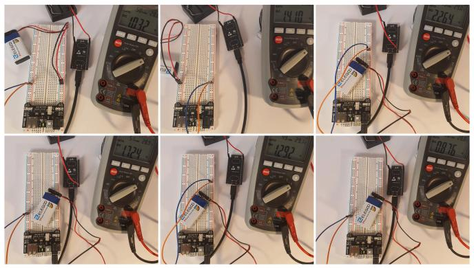
it is shown how we tried to work on many schematics using the 3V3 volts in the power supply or the 5V. The power supply is linked to the ESP32 using a micro cable USB or the 5V pin as an input. When using the micro cable USB, also we had two options, one to use the pin 3V3 as output in the ESP32, and the other to use the pin 5V. In all options, the maximum voltage supplied from the ESP32 to the sensors was 2.2 volts, which is also insufficient to power our sensors.
