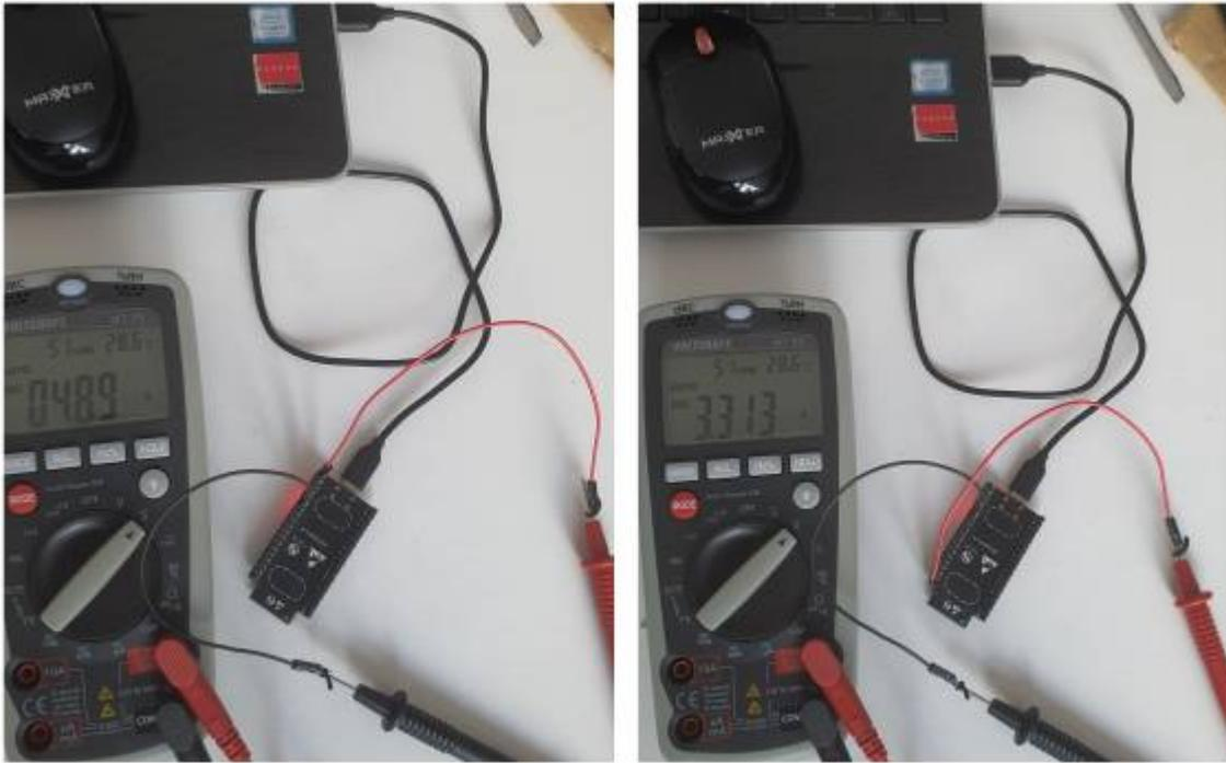
**Figure 19** Measuring the voltage supplied by the Laptop USB port from the pins 5V and 3V3
