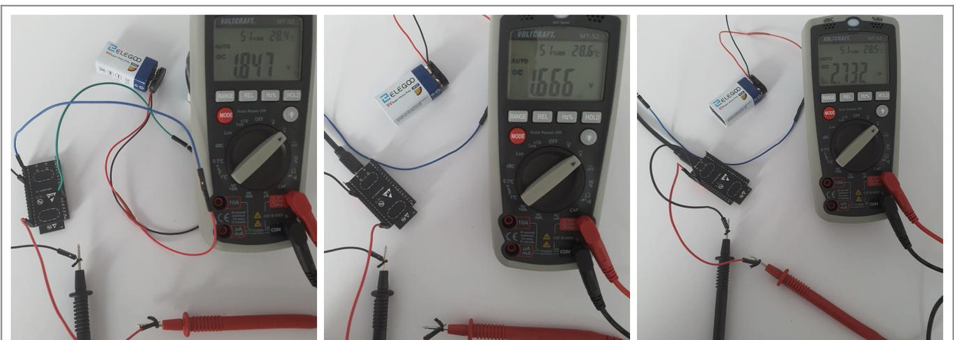
**Figure 17** Collage of trials connecting the battery using the micro cable USB as input and the 5V pin as output.
