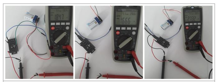
**Figure 19** Collage of trials connecting the battery using the micro cable USB as input and the 5V pin as output.
