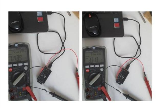
Figure 21 Measuring the voltage supplied by the Laptop USB port from the pins 5V and 3V3
