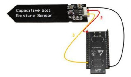
Figure 3 Connection of the Capacitive Soil Moisture with the ESP32, Picture by: Ziad Helou
