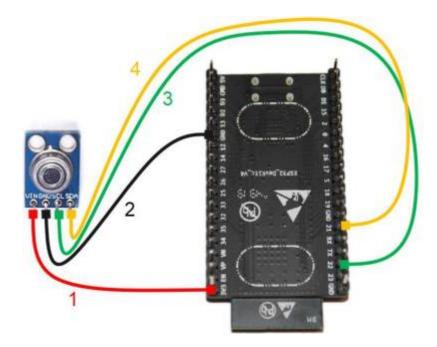
**Figure 4** Connection of the Infrared temperature sensor with the ESP32, Picture by: Ziad Helou
