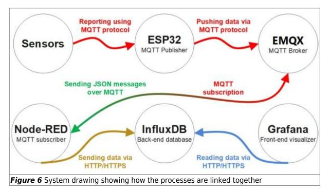
Sensors must be configured to send data reports using MQTT. Each sensor is a client and connects to the MQTT server under a specific topic.
