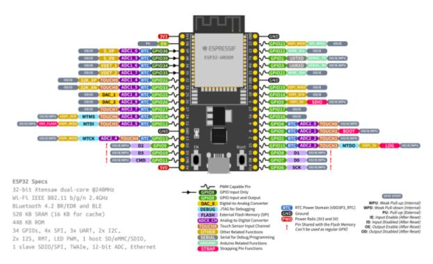
Figure 1 Pin layout detailed of the ESP32-DevkitC microcontroller.
