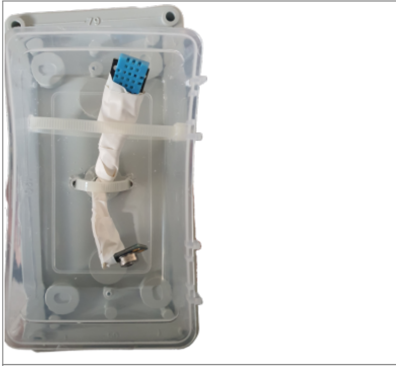
Figure 10 Sensors being covered with protective material
