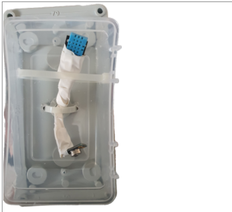
Figure 10 Sensors being covered with protective material
