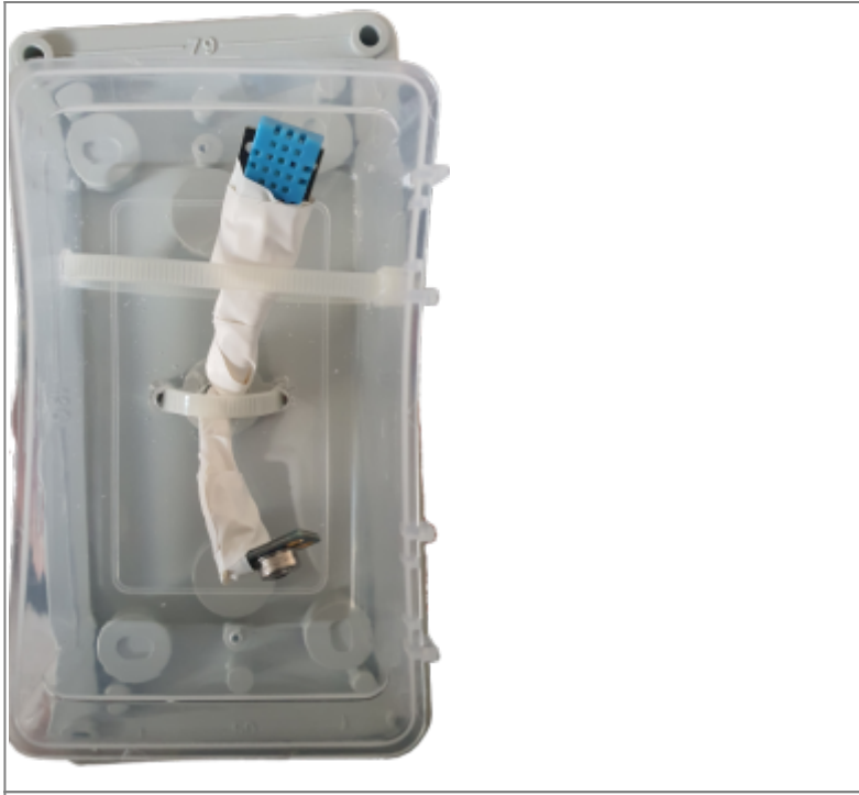
Figure 10 Sensors being covered with protective material
