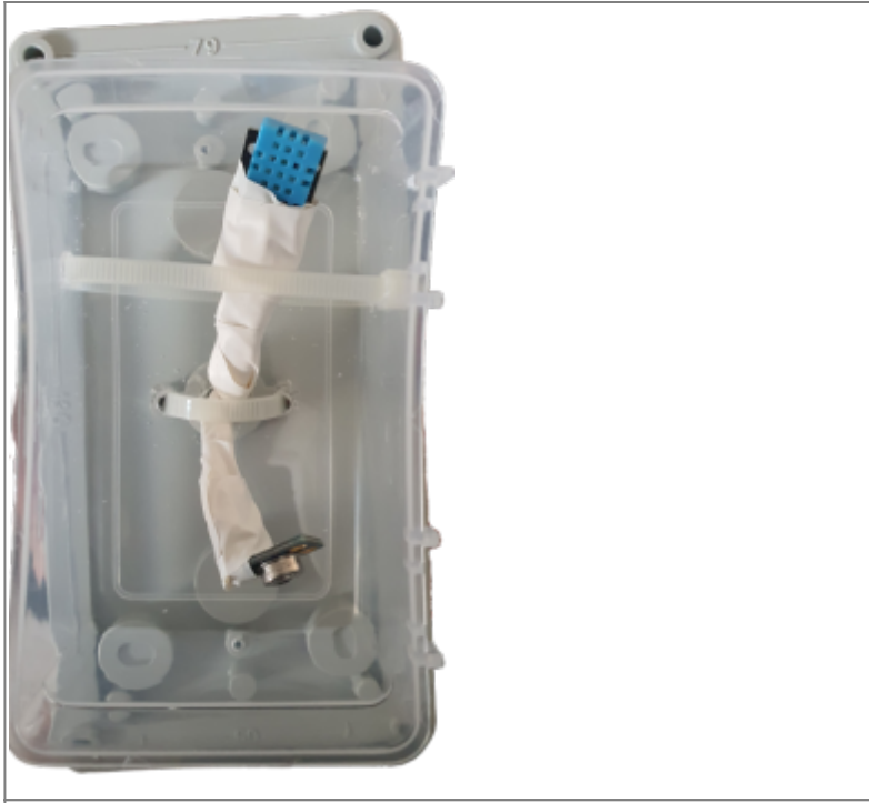
Figure 10 Sensors being covered with protective material
