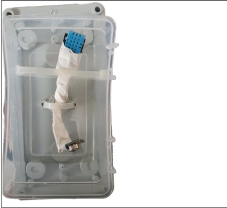
**Figure 10** Sensors being covered with protective material
