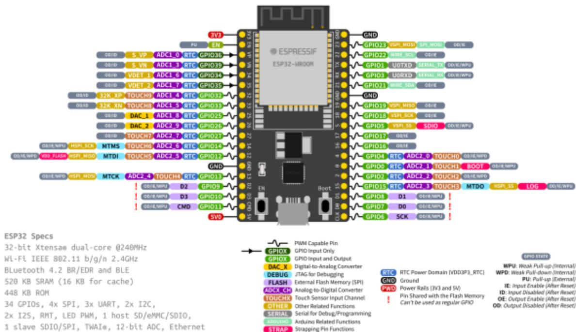
**Figure 1** Pin layout detailed of the ESP32-DevKitC microcontroller.
