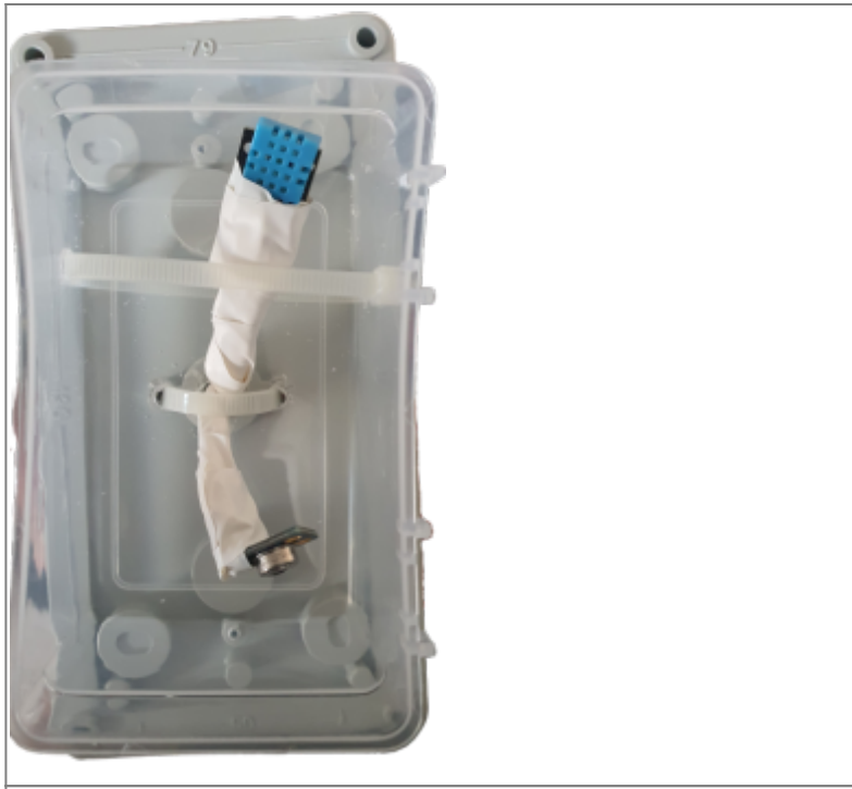
Figure 10 Sensors being covered with protective material
