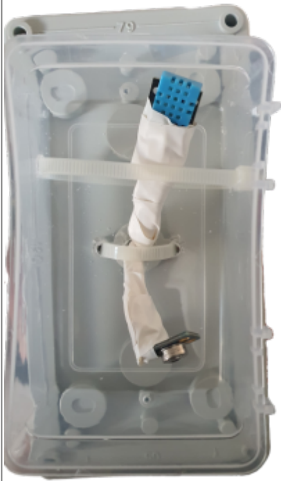
Figure 10 Sensors being covered with protective material, Photo by Ziad Helou
