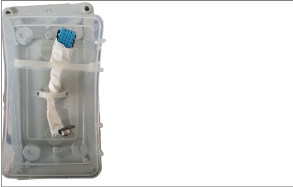
Figure 10 Sensors being covered with protective material, Photo by Ziad Helou
