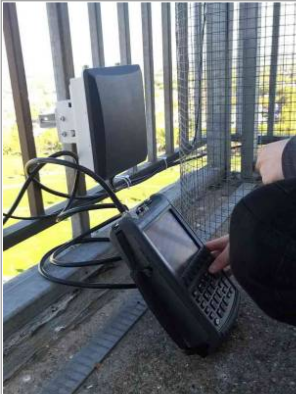
Fig.: Using a vector network analyzer to tune the antenna performance.
