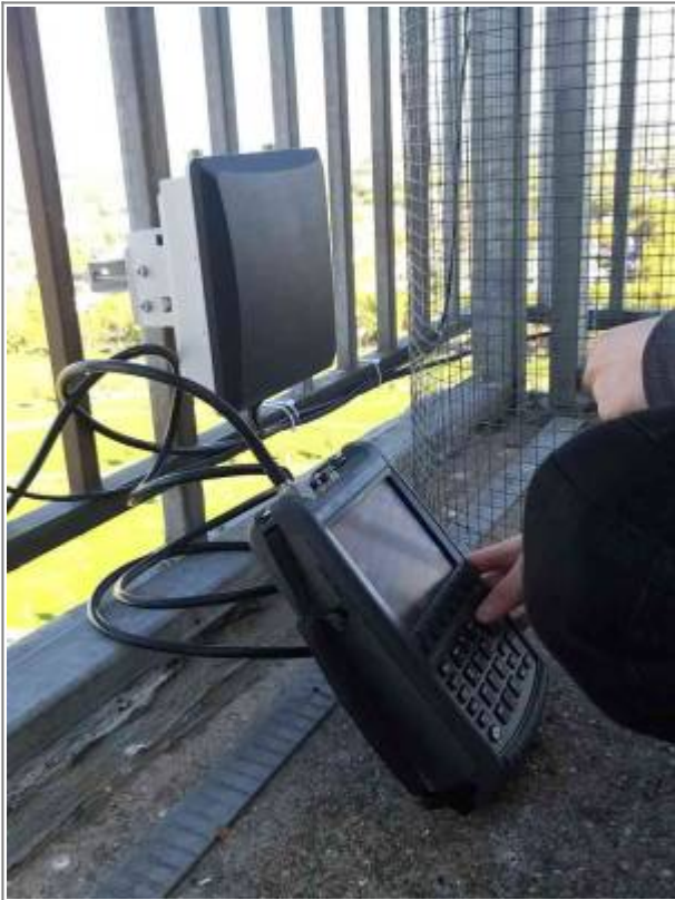
Fig.: Using a vector network analyzer to tune the antennae performance.
