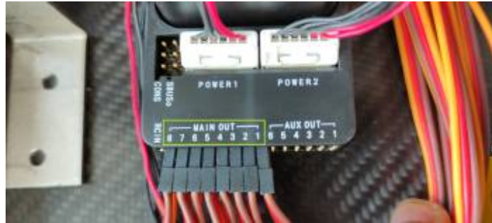
Image: Pixhawk output pins. Source: https://ardupilot.org/copter/docs/connect-escs-and-motors.html#
