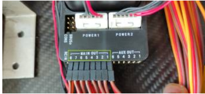
Image: Pixhawk output pins. Source: https://ardupilot.org/copter/docs/connect-escs-and-motors.html#
