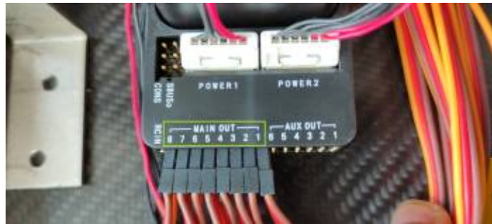
Image: Pixhawk output pins. Source: https://ardupilot.org/copter/docs/connect-escs-and-motors.html#
