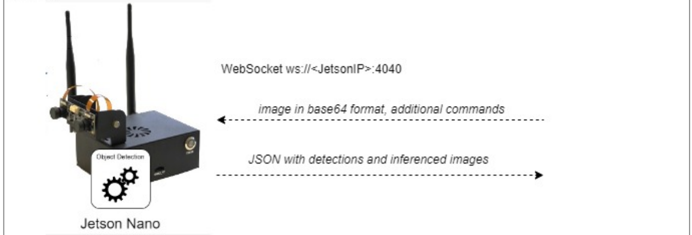
Communication diagram to Jetson device
