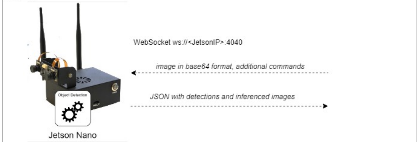
Communication diagram to Jetson device
