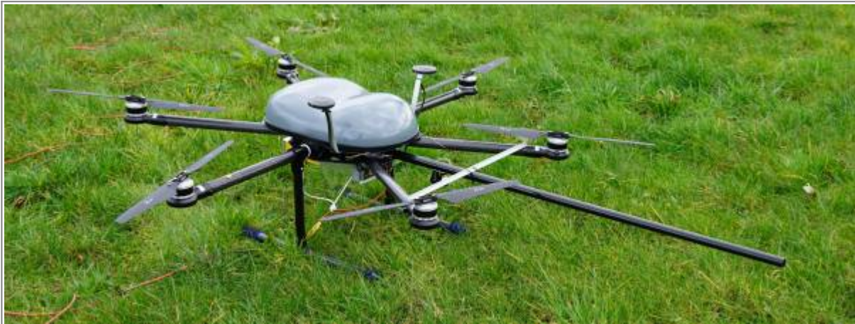
Fig.: Utility drone equipped with sprayer unit.
