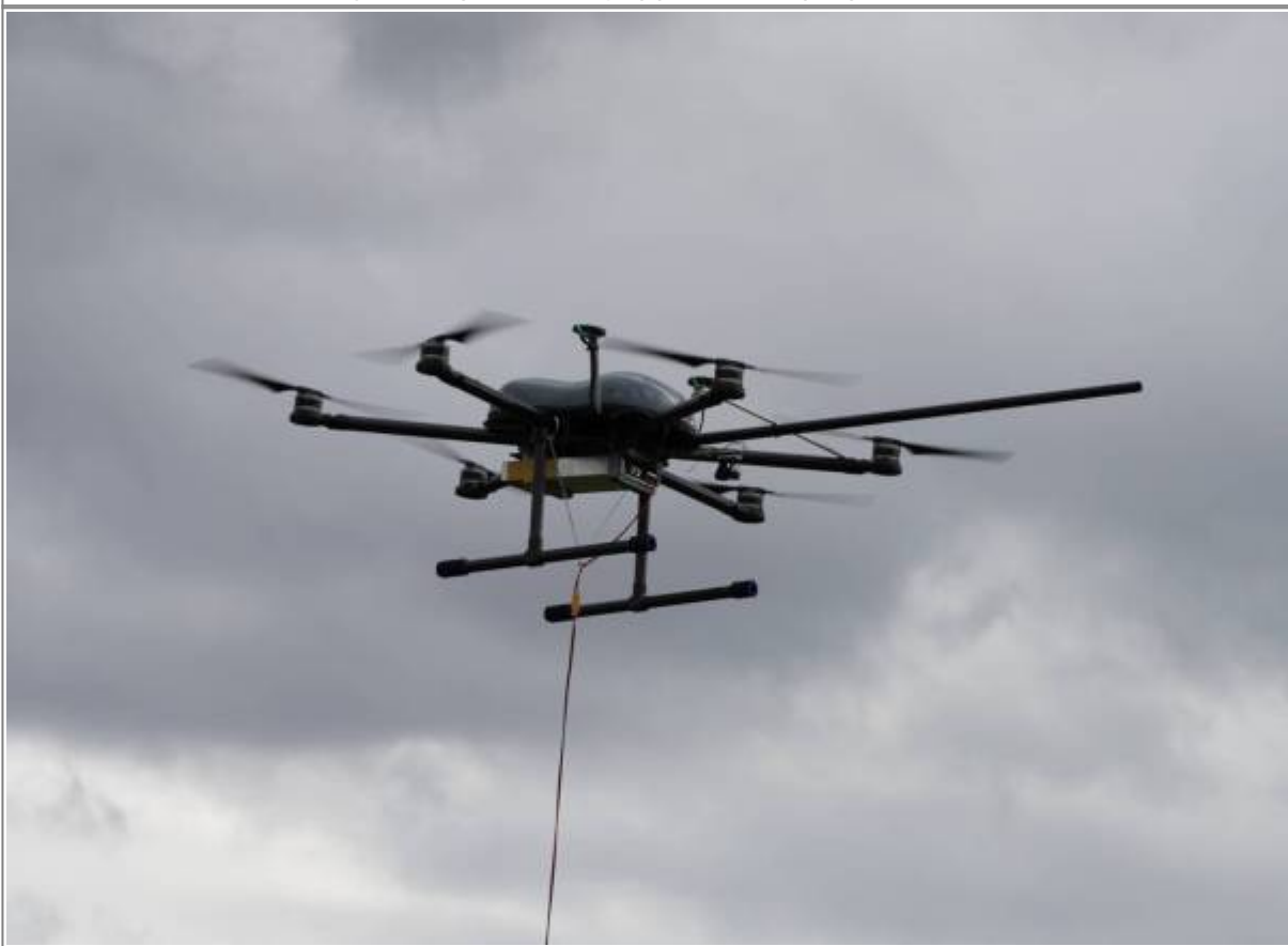
Fig.: Tethered utility drone.
