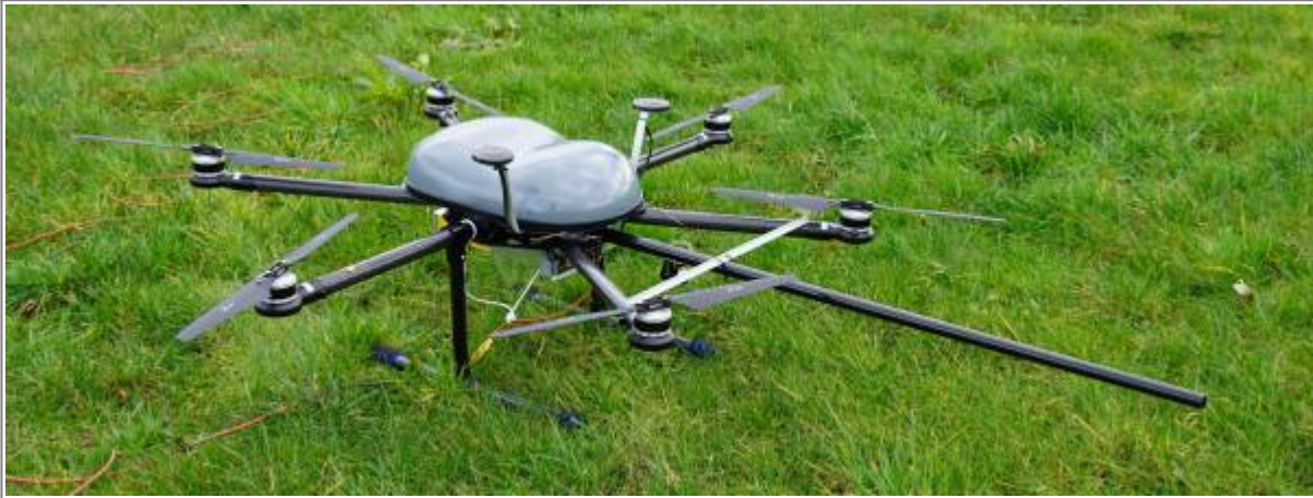
Fig.: Utility drone equipped with sprayer unit.
