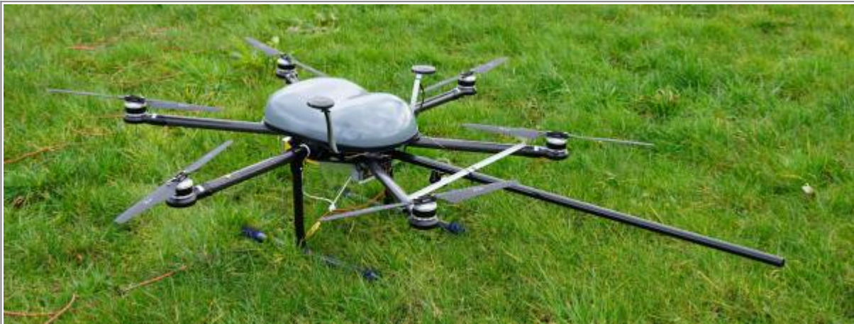
Fig.: Utility drone equipped with sprayer unit.
