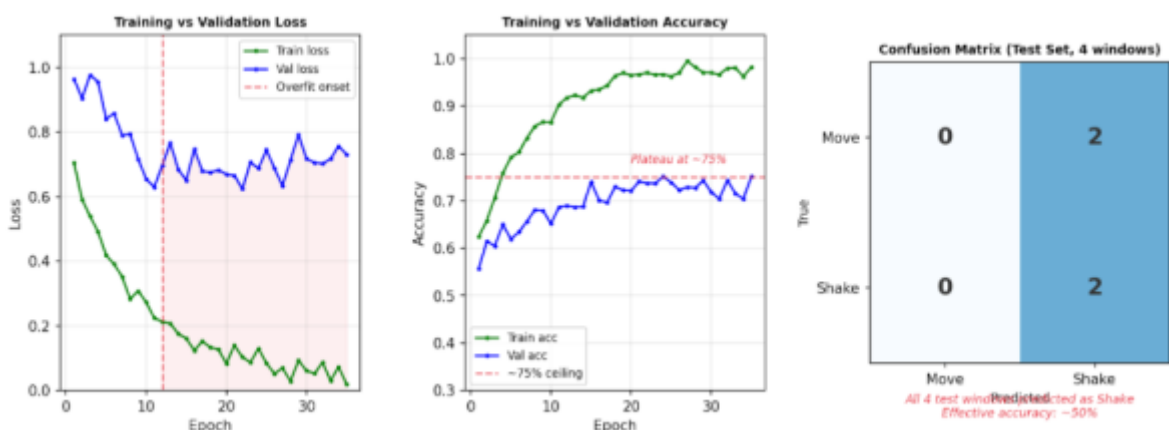
Figure 18 Model v1 training results — loss (left), accuracy (centre), and confusion matrix (right, 4-window test set). Val loss rises from epoch 12 (overfitting); all test predictions collapse to Shake.
