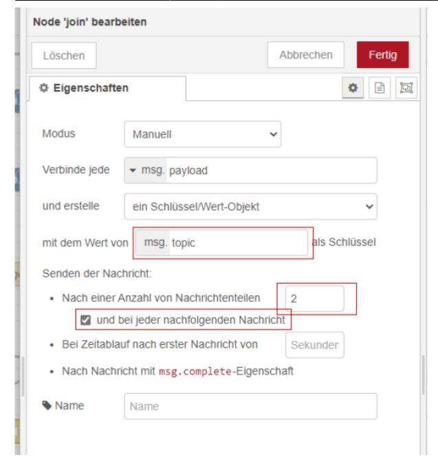
Figure 31: Properties of the join node
