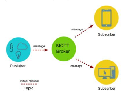
Figure 2: Structure of MQTT
