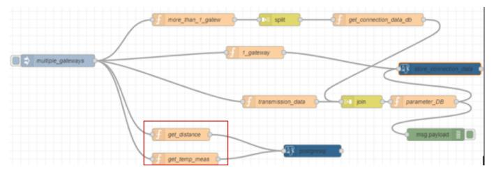
Figure 24: Functions to extract data for the measurement tables
