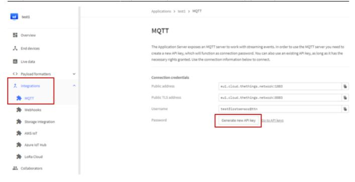
Figure 36: How to generate API key for MQTT
