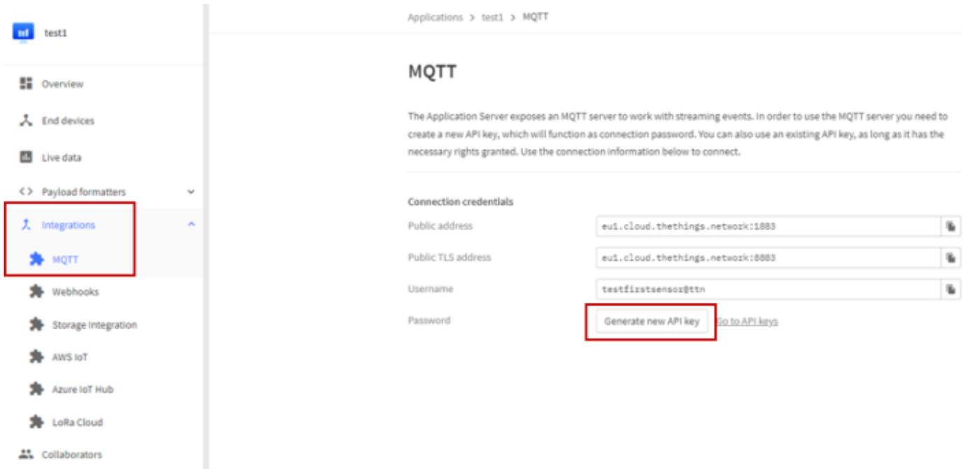
Figure 36: How to generate API key for MQTT
