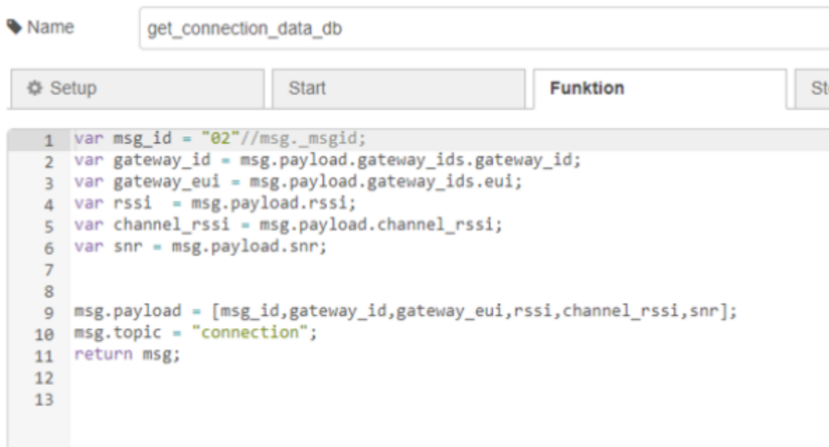
Figure 30: Details for the function "get_connection_data"
