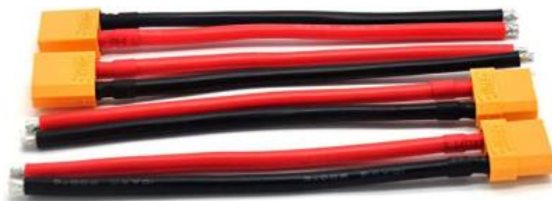
Figure 18 Soldering wires to XT60 connector
