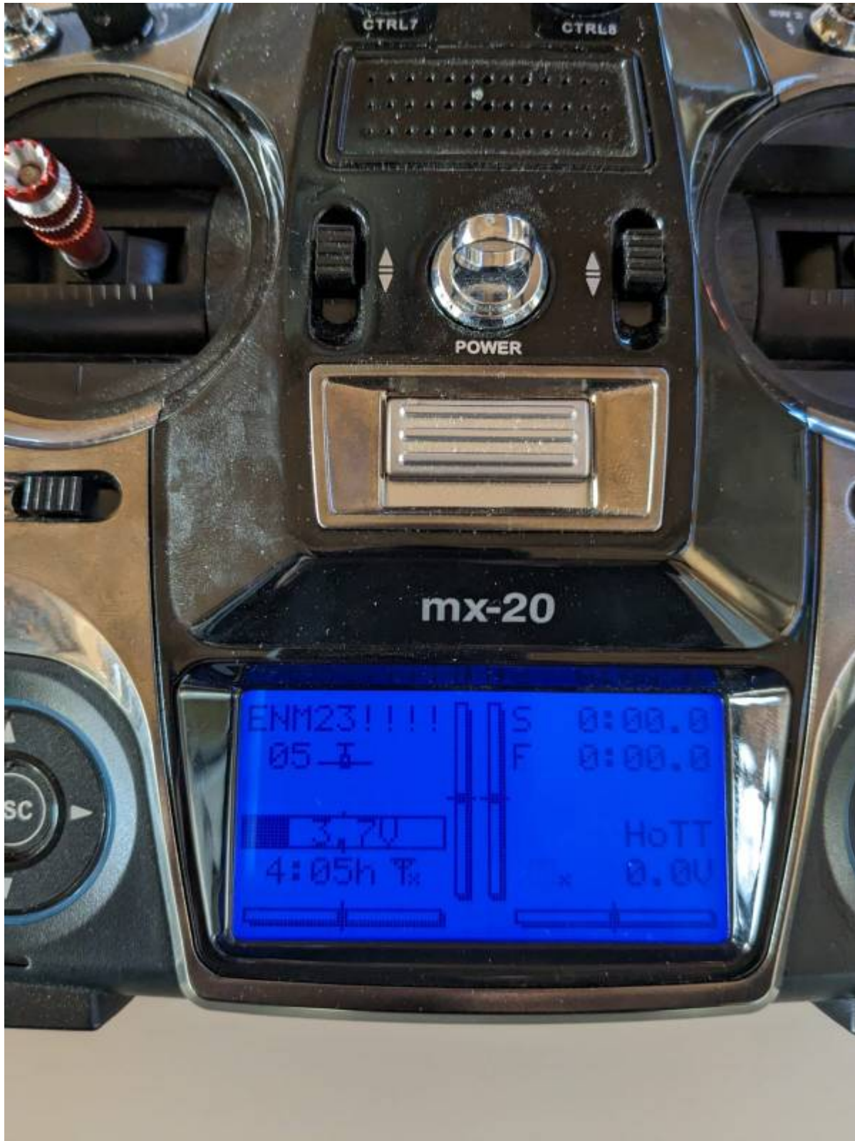
Figure 38: Graupner transmitter confirming receiver binding
