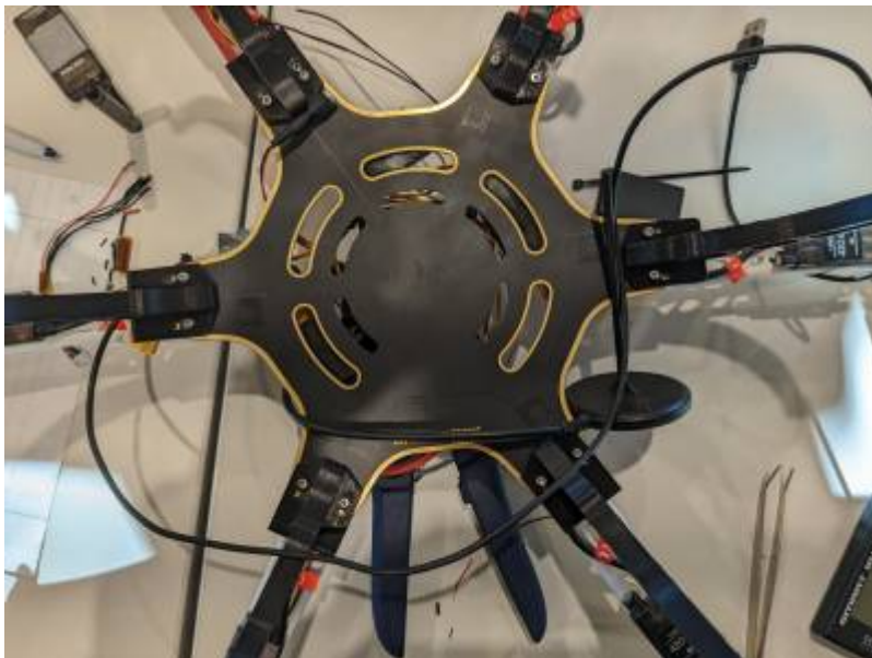
Figure 34 Adding 6 landing gear to 6 base frame
