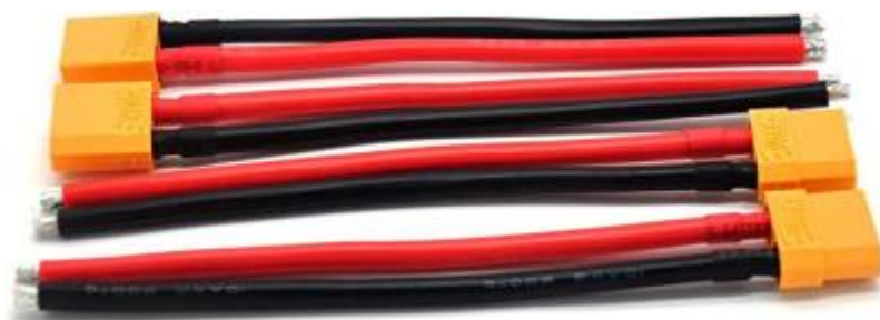
Figure 4.4 Soldering wires to XT60 connector
