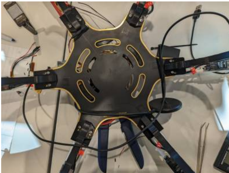
Figure 8.2 Adding 6 landing gear to 6 base frame
