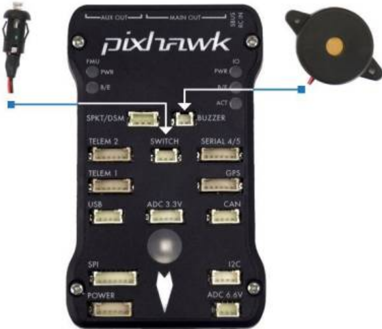
Figure 7.3 Safety switch and buzzer location and connection
