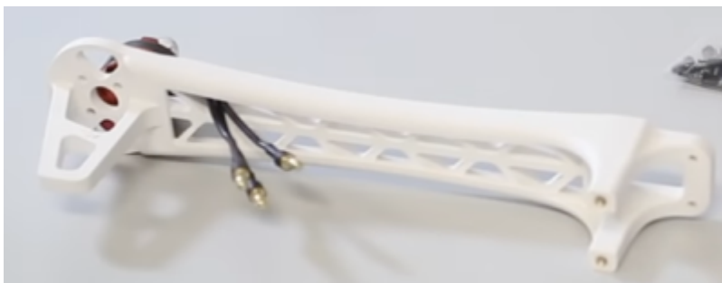
Figure 4.1 Mounting servo motor to arm
