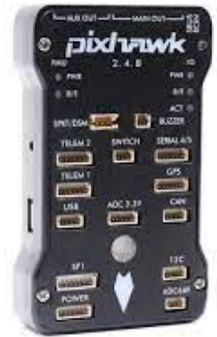
Figure 2: pixhawk 2.4.8 flight controller
