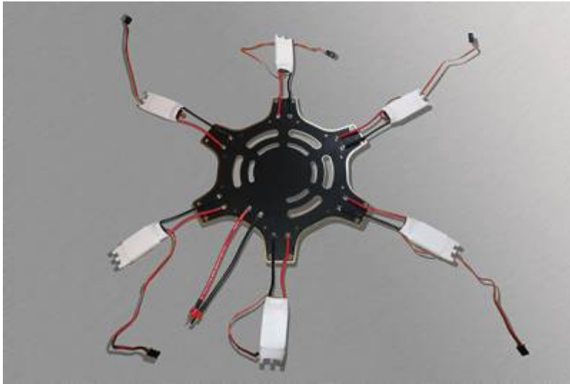
Figure 4.3 basic skeleton with all ESCs and power supply cable attached
