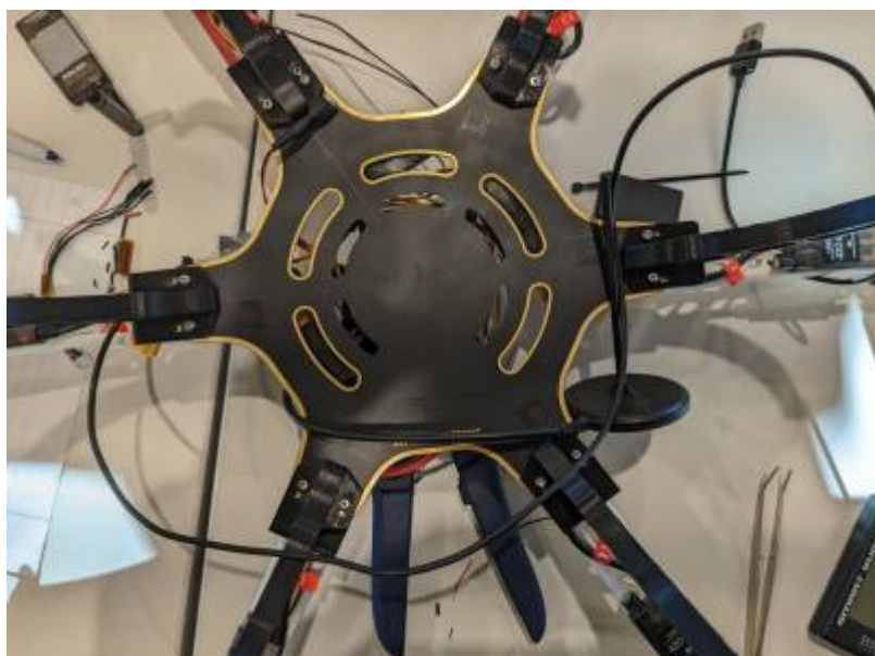
Figure 8.2 Adding 6 landing gear to 6 base frame
