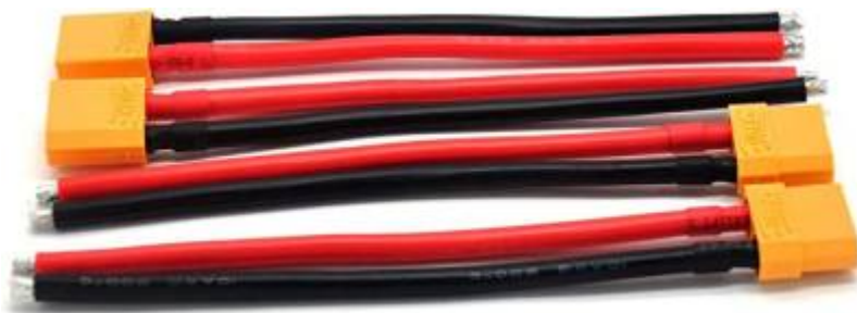
Figure 4.4 Soldering wires to XT60 connector
