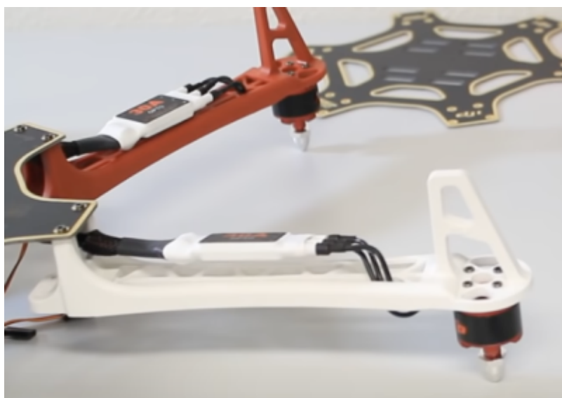
Figure 6.1 Upside down view of connecting servo motor wire to ESCs
