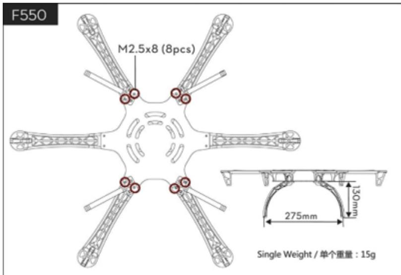
Figure 8.1 Adding 4 landing gear to 6 base frame
