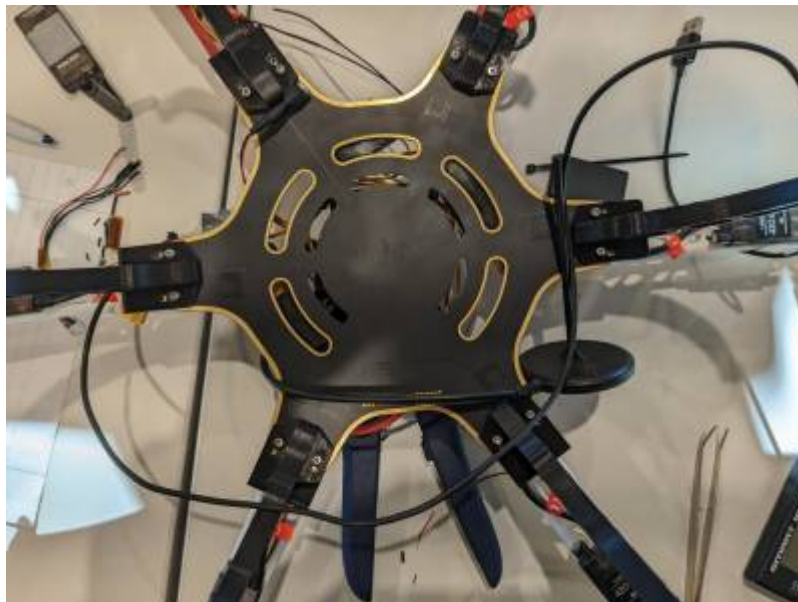
Figure 8.2 Adding 6 landing gear to 6 base frame
