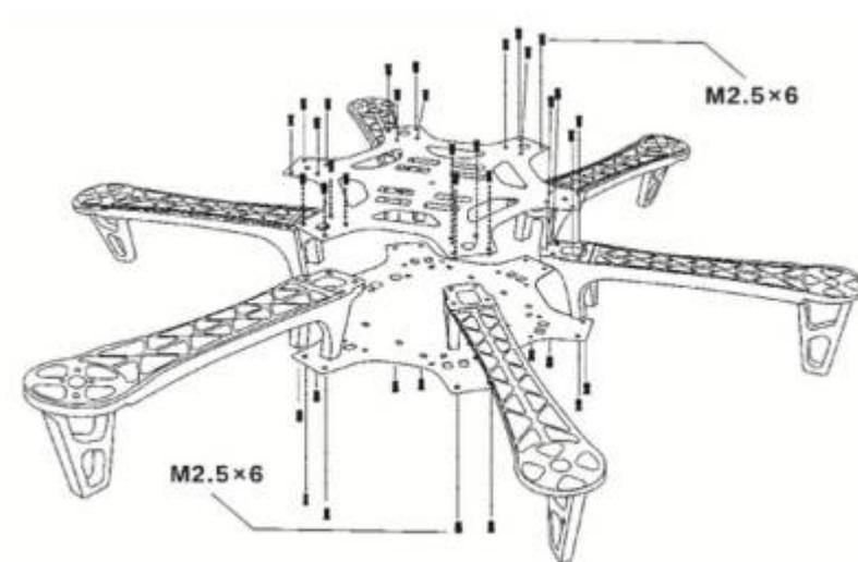
Figure 4.6 Bottom view for screw attachment to arms
