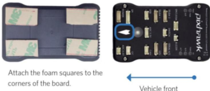
Figure 7.2 Double sided tape below the flight controller
