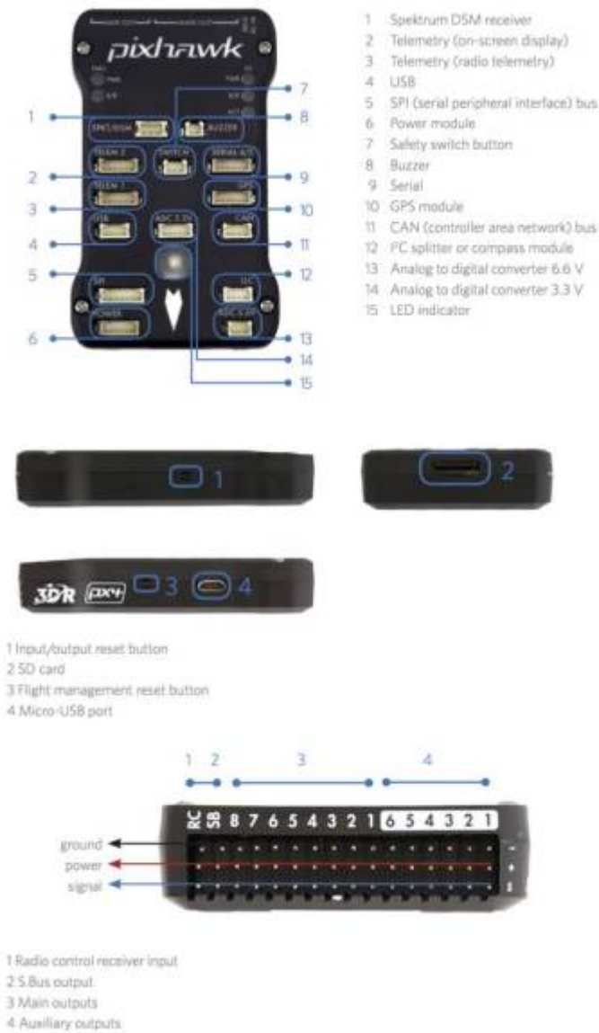
Figure 7.1 Diagram of PixHawk 2.4.8
