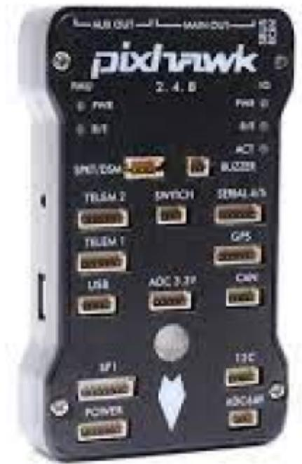
Figure 2: pixhawk 2.4.8 flight controller
