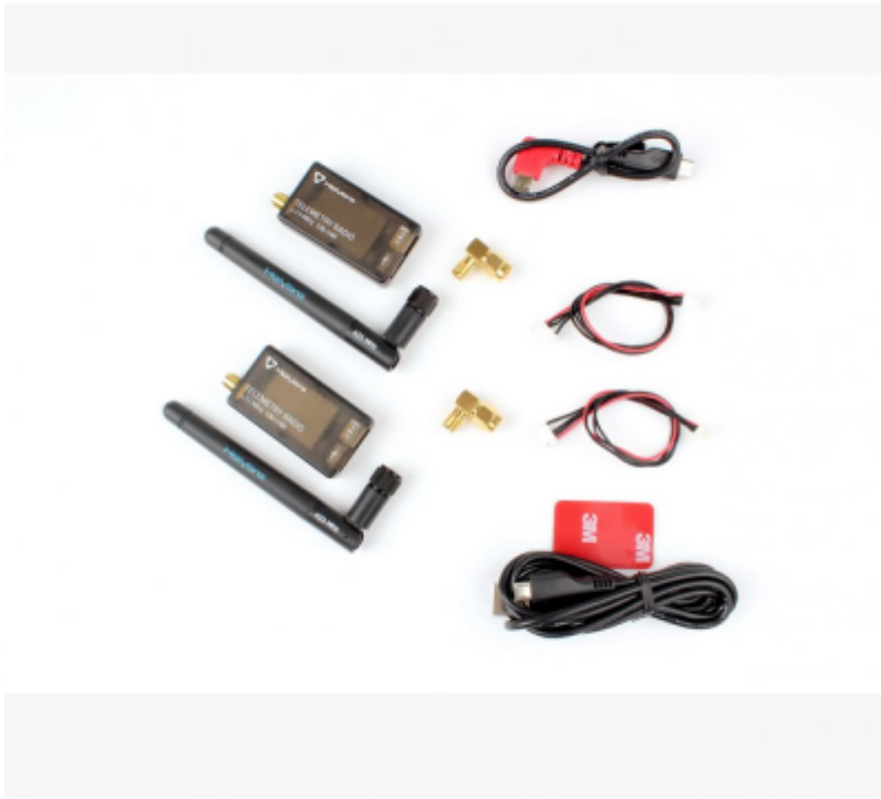
Figure 6: 433MHz Holybro telemetry radio set
