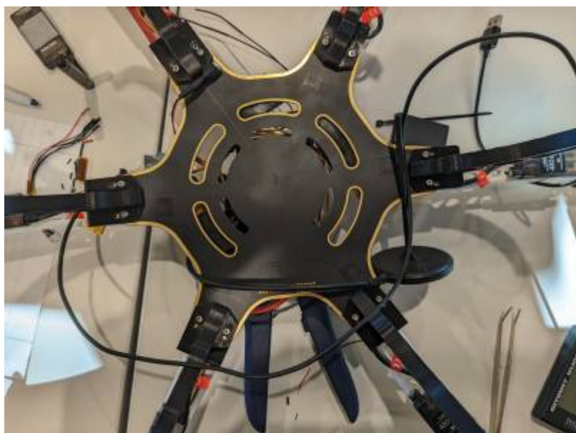
Figure 8.2 Adding 6 landing gear to 6 base frame
