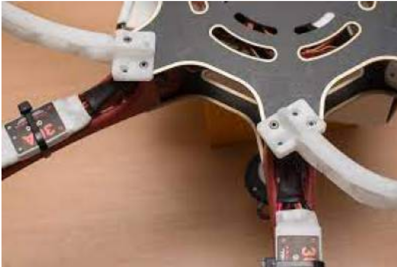
Figure 5.1 using zip ties for mounting ESCs to the arm
