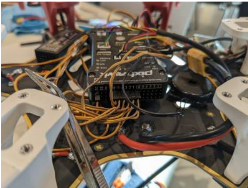
Figure 7.8 Connecting ESCs to the flight controller
