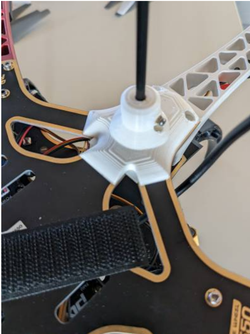
Figure 11.1 Mounting GPS unit on top frame
