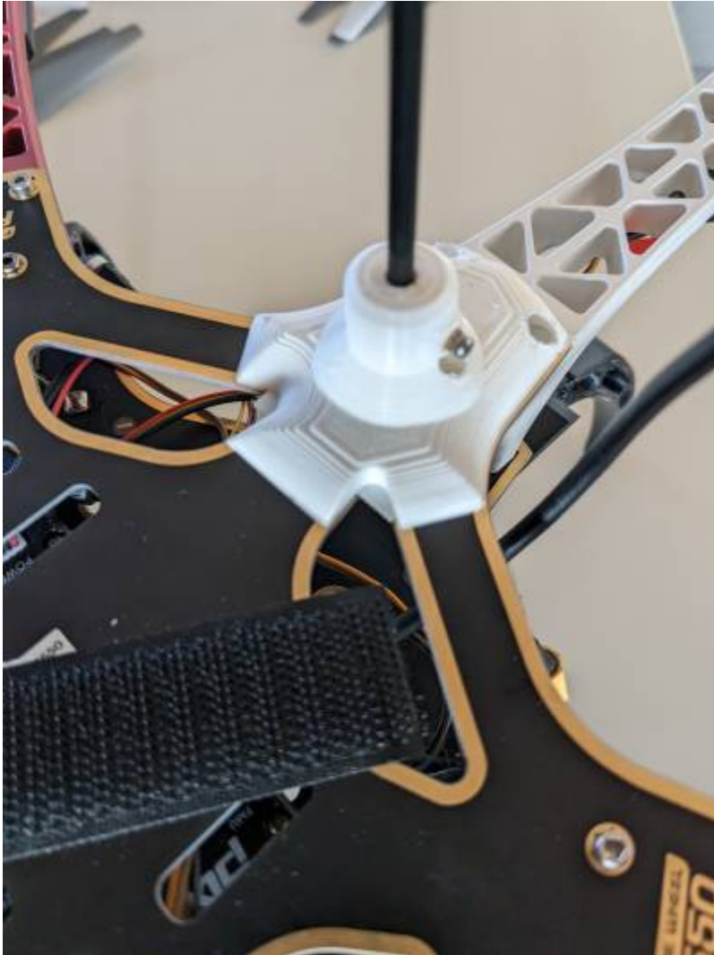
Figure 11.1 Mounting GPS unit on top frame
