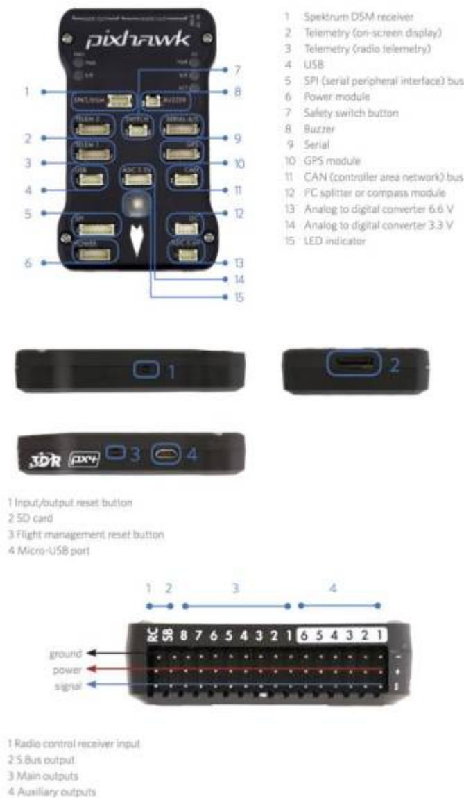
Figure 7.1 Diagram of PixHawk 2.4.8
