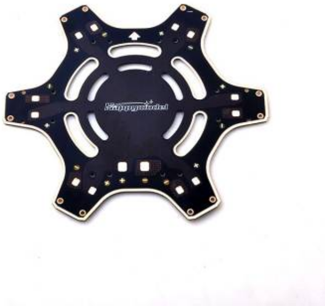
Figure 4.2 Connections with positive and negative symbols on base frame
