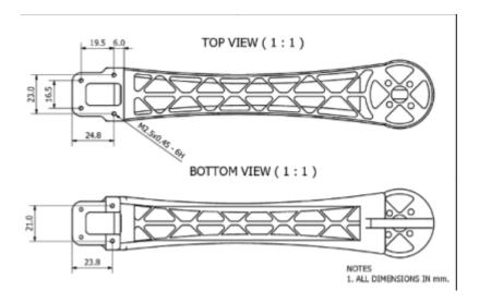
Figure 4.5 top and bottom view of the arm
