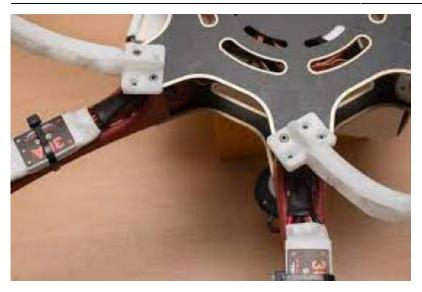
Figure 5.1 using zip ties for mounting ESCs to the arm
