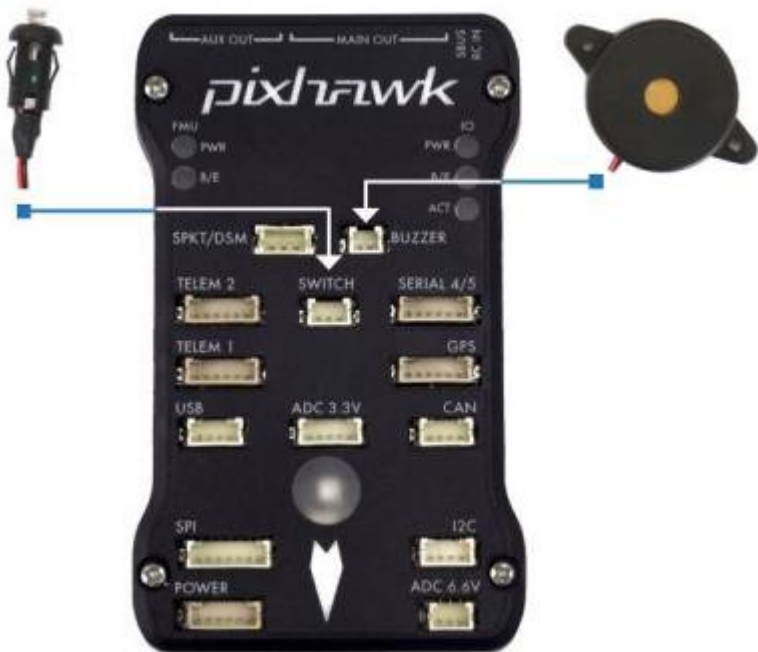
Figure 7.3 Safety switch and buzzer location and connection
