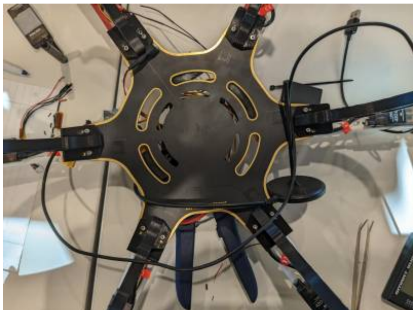
Figure 8.2 Adding 6 landing gear to 6 base frame
