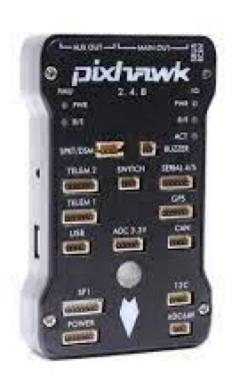
Figure 2: pixhawk 2.4.8 flight controller
