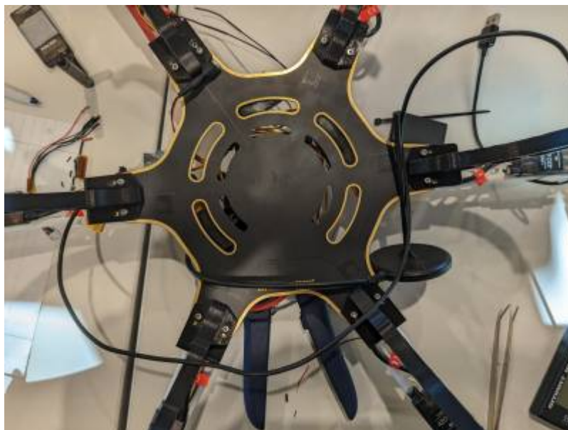
Figure 8.2 Adding 6 landing gear to 6 base frame
