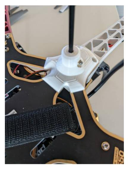
Figure 11.1 Mounting GPS unit on top frame
