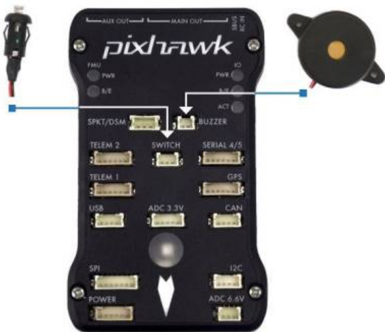
Figure 7.3 Safety switch and buzzer location and connection
