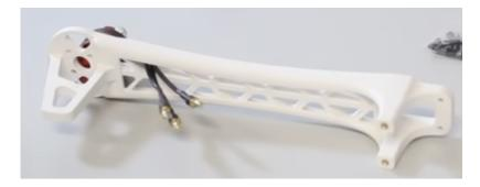
Figure 4.1 Mounting servo motor to arm
