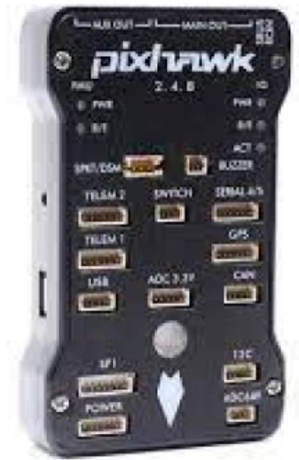
Figure 2: pixhawk 2.4.8 flight controller
