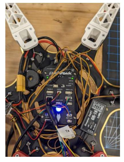
Figure 7.9 Final look for the fully connected flight controller.
