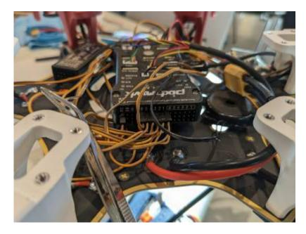
Figure 7.8 Connecting ESCs to the flight controller
