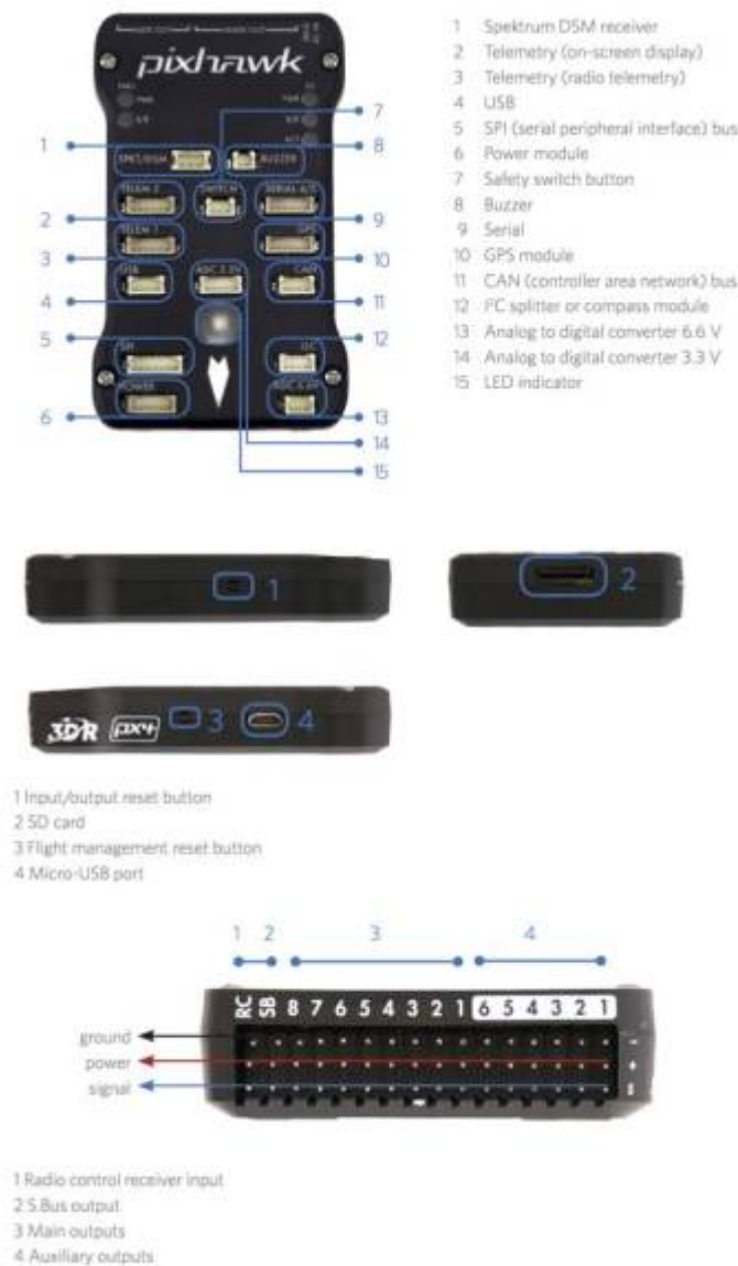
Figure 7.1 Diagram of PixHawk 2.4.8
