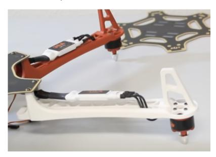
Figure 6.1 Upside down view of connecting servo motor wire to ESCs
