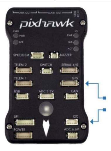
Figure 7.4 Mounting GPS module and Compass to Flight controller
