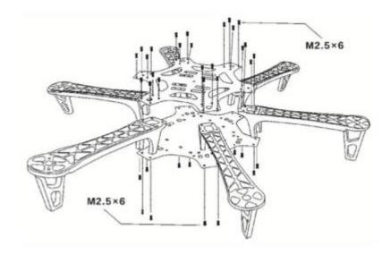
Figure 4.6 Bottom view for screw attachment to arms
