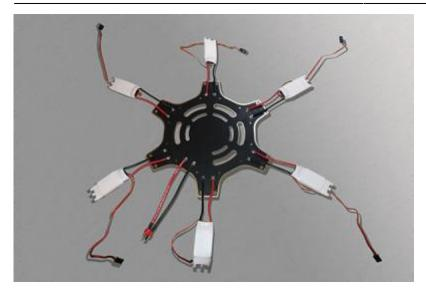
Figure 4.3 basic skeleton with all ESCs and power supply cable attached
