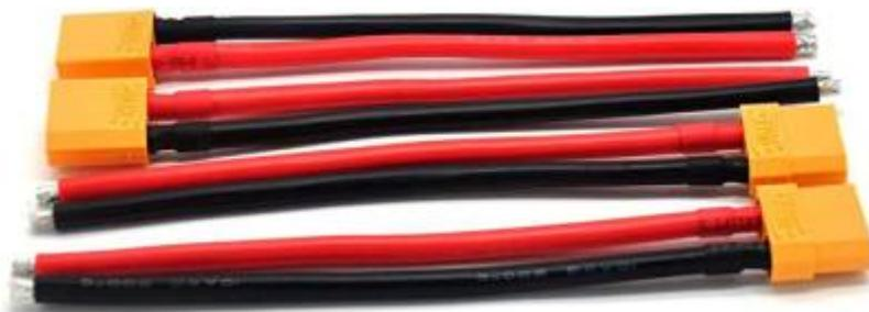
Figure 4.4 Soldering wires to XT60 connector
