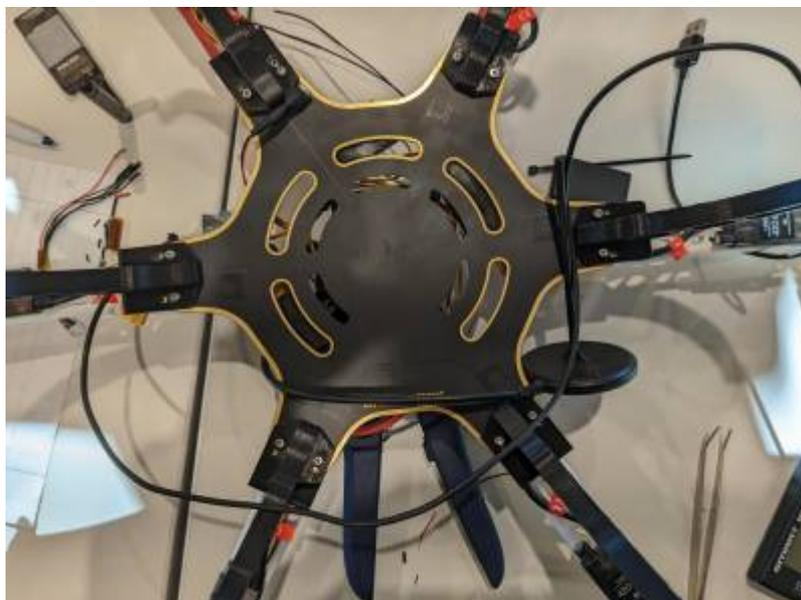
Figure 8.2 Adding 6 landing gear to 6 base frame
