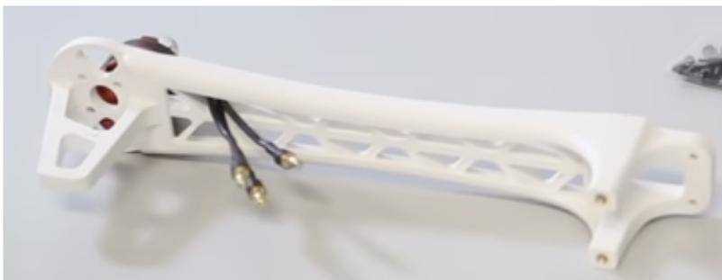
Figure 4.1 Mounting servo motor to arm
