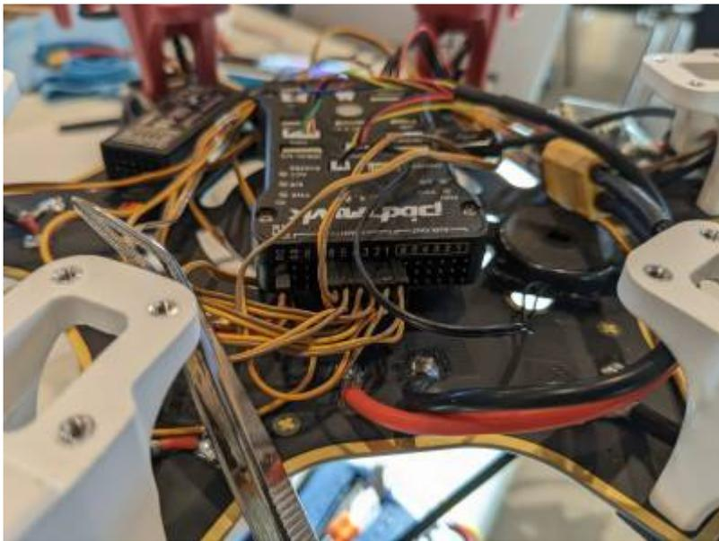
Figure 7.8 Connecting ESCs to the flight controller
