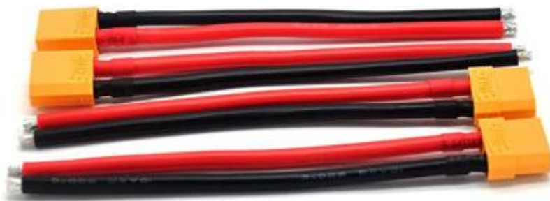
Figure 4.4 Soldering wires to XT60 connector
