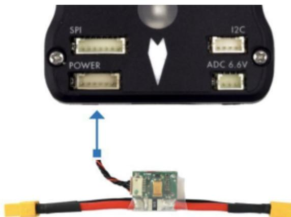
Figure 7.5 mounting power module in power socket of flight controller
