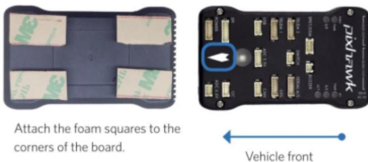
Figure 7.2 Double sided tape below the flight controller
