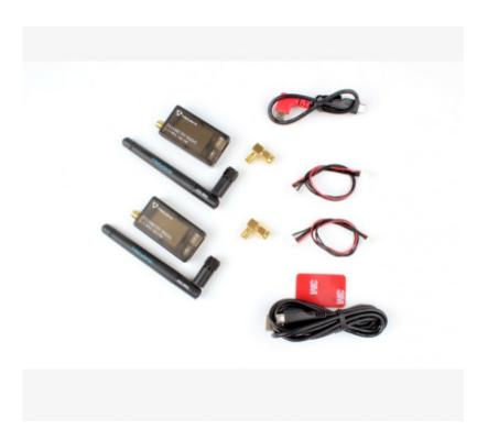
Figure 6: 433MHz Holybro telemetry radio set
