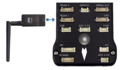
Figure 7.7 Telemetry radio to flight controller
