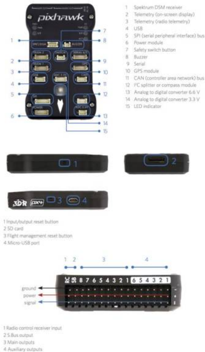
Figure 7.1 Diagram of PixHawk 2.4.8
