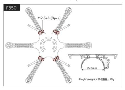
Figure 8.1 Adding 4 landing gear to 6 base frame
