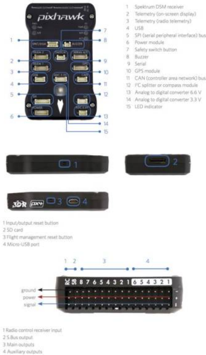
Figure 7.1 Diagram of PixHawk 2.4.8
