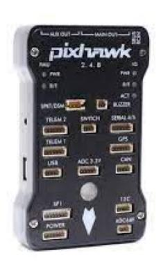
Figure 2: pixhawk 2.4.8 flight controller
