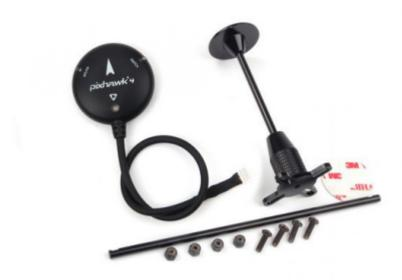
Figure 9: Pixhawk 4 GPS module
