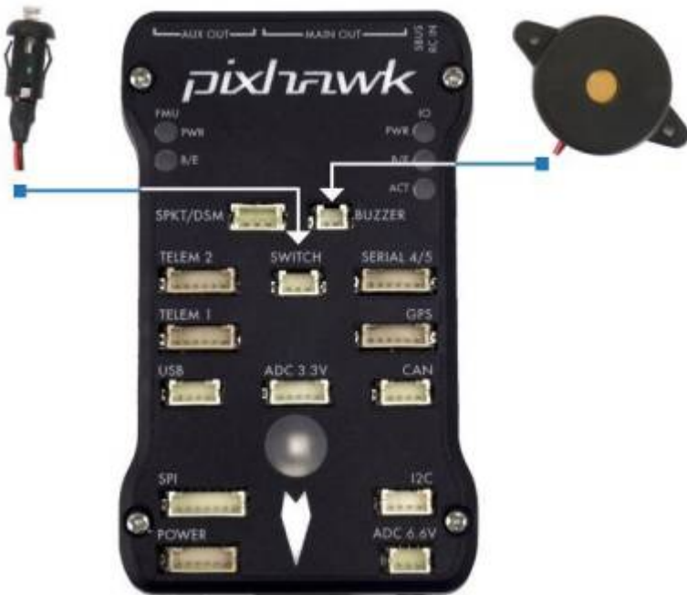
Figure 7.3 Safety switch and buzzer location and connection
