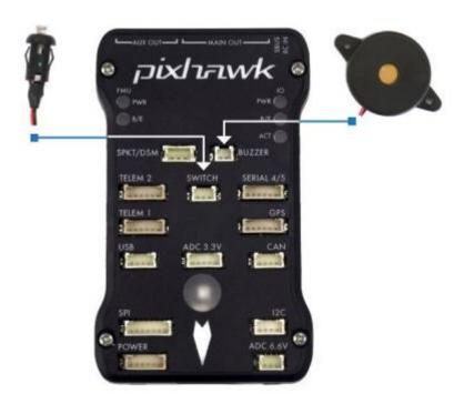
Figure 7.3 Safety switch and buzzer location and connection
