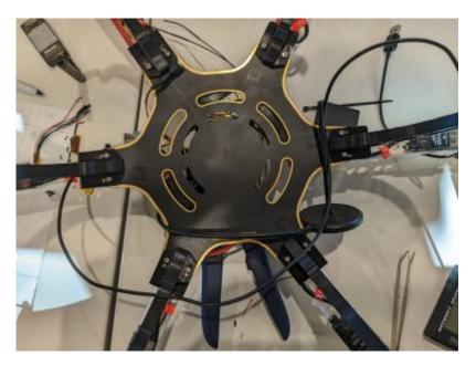
Figure 8.2 Adding 6 landing gear to 6 base frame
