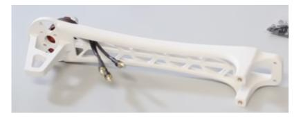
Figure 4.1 Mounting servo motor to arm
