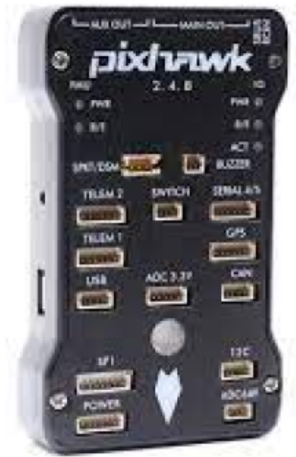
Figure 2: pixhawk 2.4.8 flight controller
