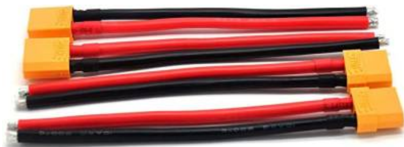
Figure 4.4 Soldering wires to XT60 connector
