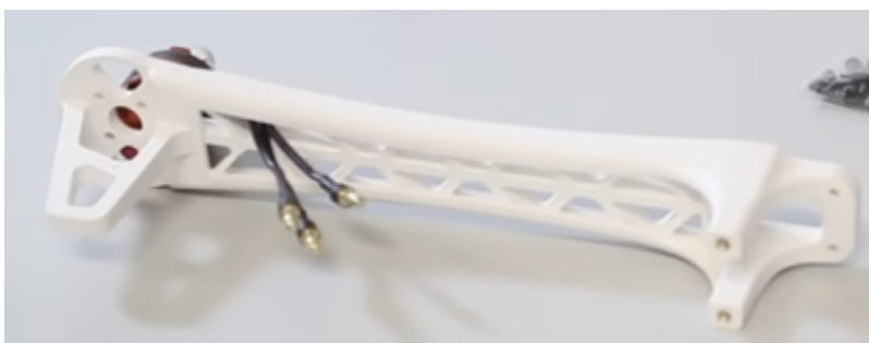
Figure 4.1 Mounting servo motor to arm
