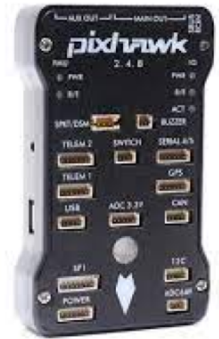
Figure 2: pixhawk 2.4.8 flight controller
